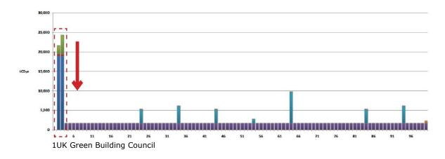
The illustration shows the  $CO_2$  emissions of an office building with a life span of 100 years. Most of the emissions are caused in the first two years during construction. The largest  $CO_2$  reduction can be achieved by looking at the choice of materials and the construction process. The constant  $CO_2$  emissions take place through the use of gas and electricity. In addition, there are a number of peak moments when a lot of  $CO_2$  is emitted due to necessary maintenance.
